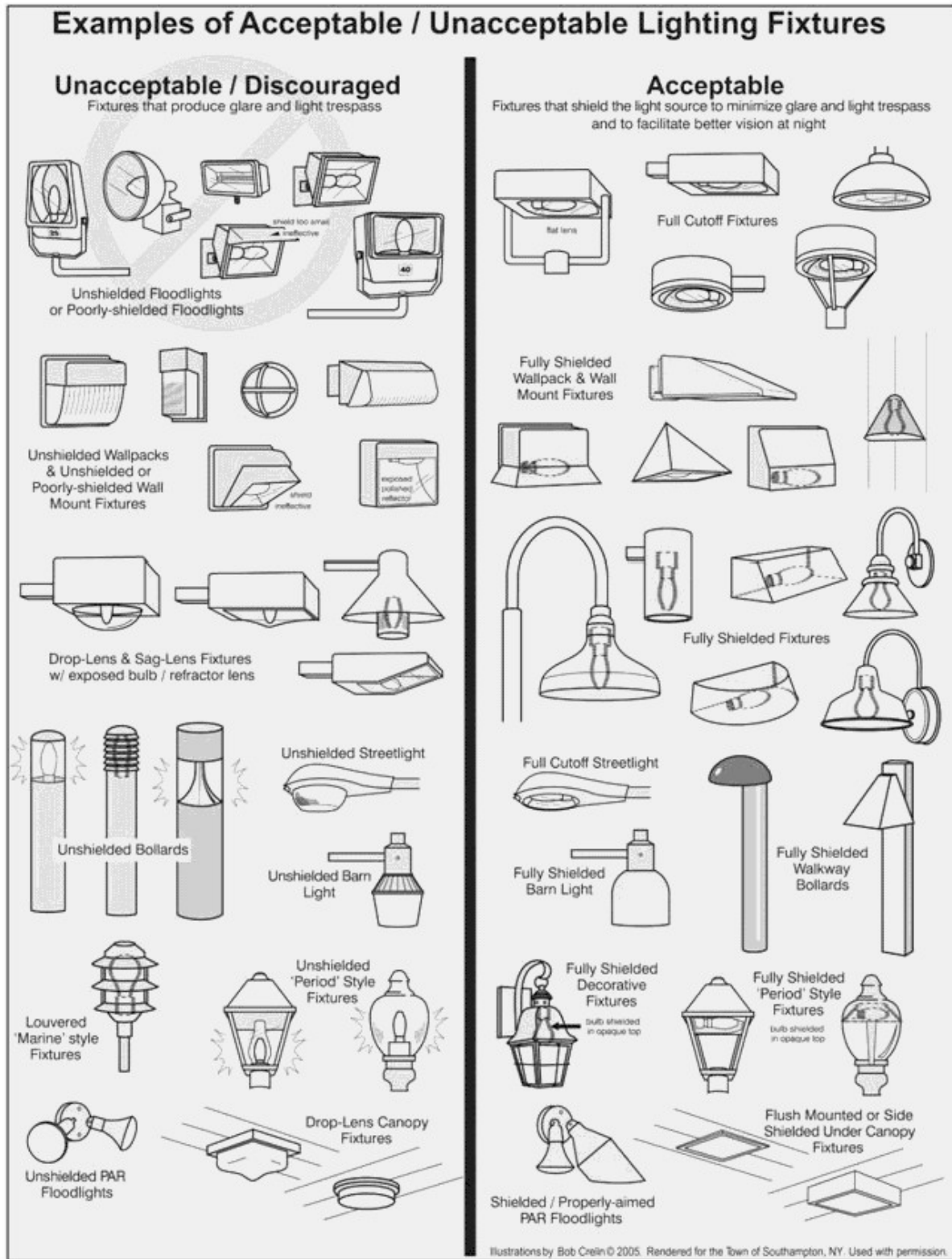
Figure 04-2: Full Cutoff Light Fixture Examples 165
