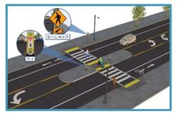
Figure 18. Pedestrian Crossing Road Diet Example
