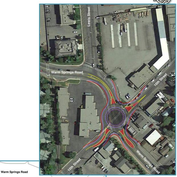
Figure 15. Warm Springs Road and 10th Street Single Lane Roundabout Concept
