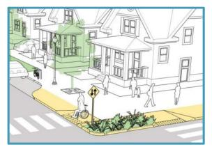
Figure 19. Bulb Out Example
